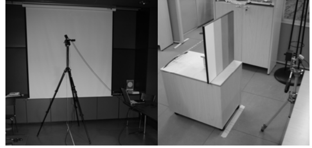
Figure 1. Test setups: measurement of the silver screen (left) and the 4-step Spectralon reference panel (right).
