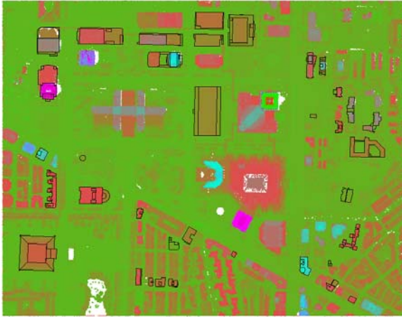
Figure 8. Point clouds with building boundaries of Case II The top-view and perspective-view of reconstructed DBM is shown in Figure 9. After including the interior roof structure, the number of building polygons increased further from 158 to 557. A comparison of vector maps with the generated building models showed that the models preserve more detail than the vector maps. The flat roof was the simplest shape and with the largest number of 262. This area contains 7 slant, 30 gable, 9 camber and 2 sphere roofs. The result indicated that the non-flat roofs were split into many small polygons to represent the non-linear roof tops. For example, two sphere roofs were split into 149 small polygons.
