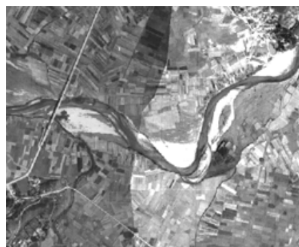
Figure 5. the mosaicked image without seamline removing
