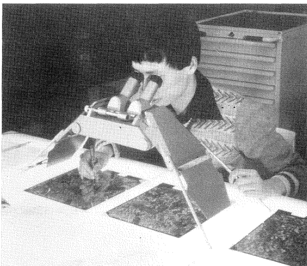
Fig. 5 Stereoscope, a standard instrument for photo-interpretation.
